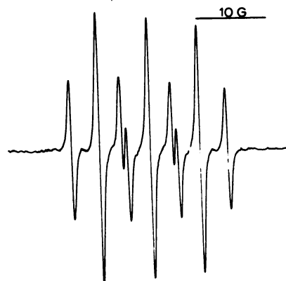
FIG. 3. The electron spin resonance spectrum obtained when 1-hydroxyl-5,5-dimethylpyrrolid-2-one is oxidized by a variety of one electron sources
